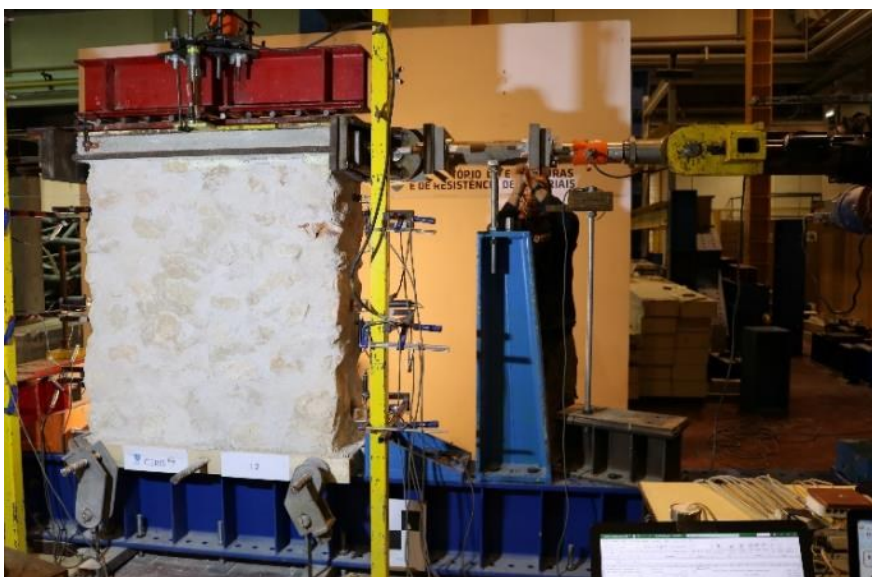
Quasi-static cyclic test setup on a rubble stone wall.
