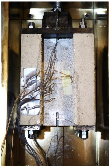
CFRP-concrete bond test at elevated temperature.
