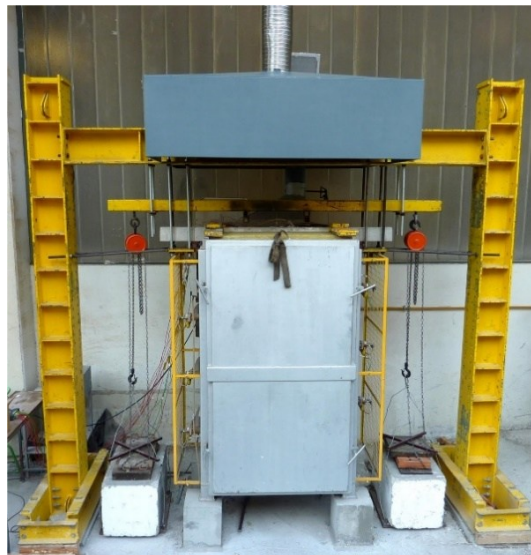
Fire resistance test setup.
