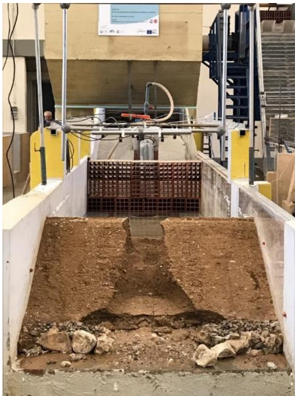
Dam breach by overtopping. Experimental test.
