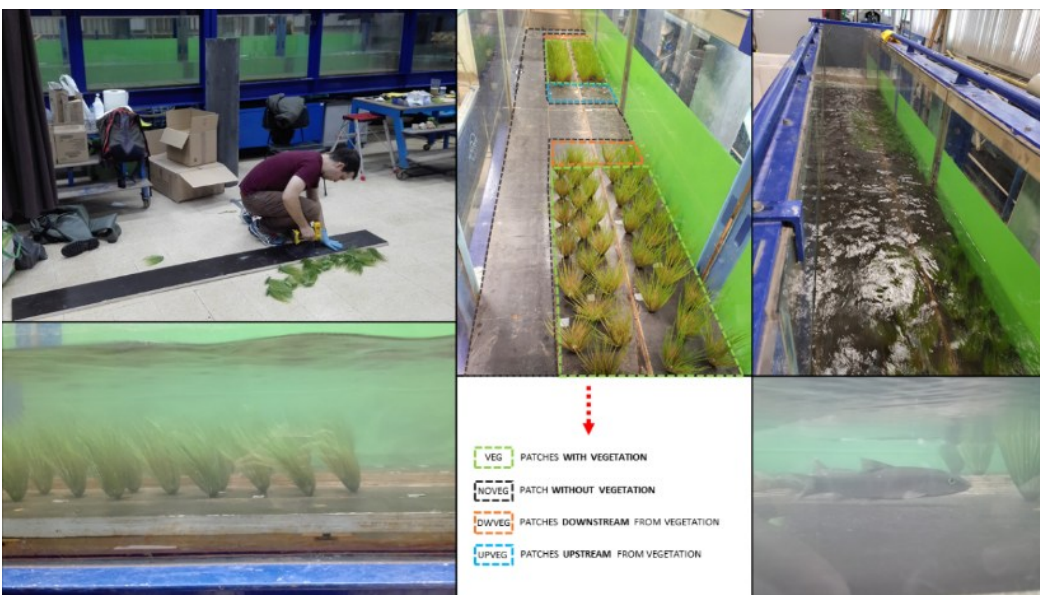
Flow field properties and fish occupation of 1) patches with plants (VEG, green dotted rectangles); 2) patches upstream (UPVEG, blue dotted rectangle) and 3) downstream (DWVEG, orange dotted rectangles) from vegetation; and 4) patches without vegetation (NOVEG, black dotted area) were measured to assess sheltering behavior of L. bocagei and P. polylepis under baseflow and hydropeaking scenarios. Plants generated lower current velocity, lower hydrodynamic pressure and lower turbulence inside vegetated areas and downstream from plants, promoting hydraulically stable zones for fish to shelter.
