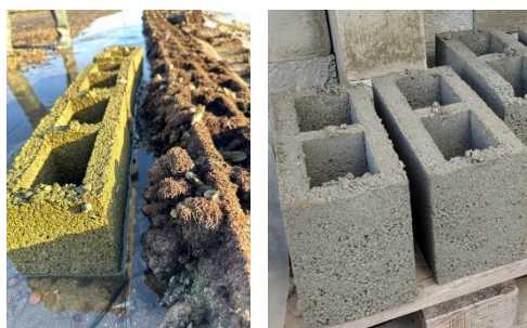
Figure 2. Ecological concrete blocks made with oyster shell waste.
