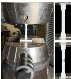
Figure 1. Material characterisation tests of high-strength steels (with video extensometer).
