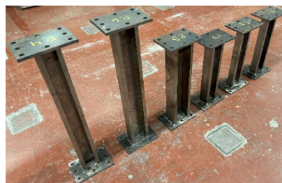
Figure 2. High-strength cold-formed steel profiles (C-sections).
