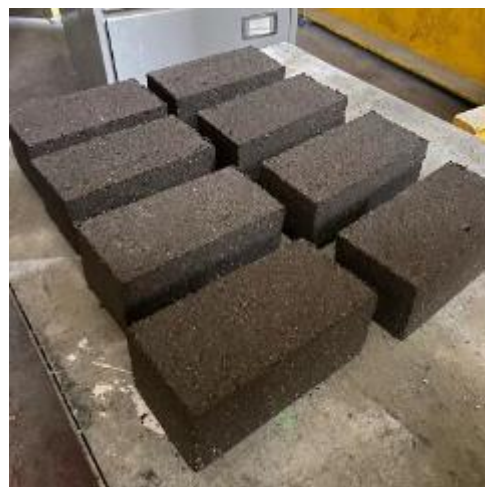
Figure 1. Alkali-activated concrete pavement blocks after an accelerated carbonation curing regimen.
