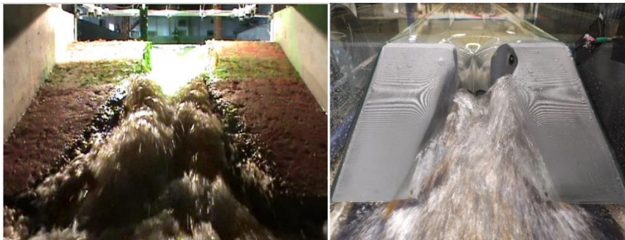
Figure 1. Breaching of overtopped dams. Left: physical model; right: fixed bed model to investigate hydrodynamic processes.
