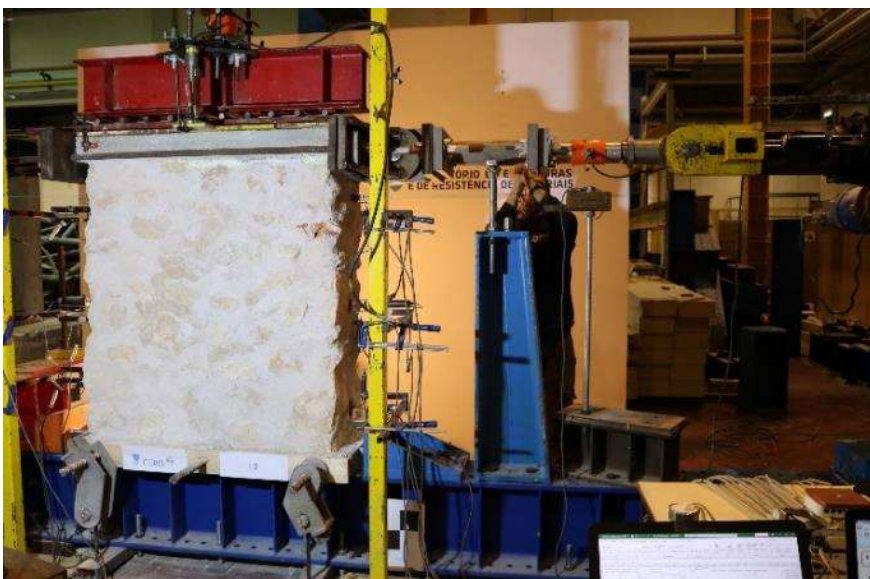
Quasi-static cyclic tests setup on a rubble stone wall.
