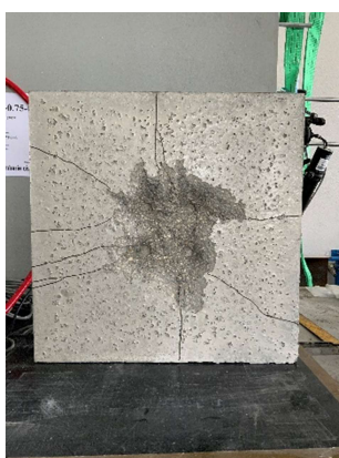
Anchor strength: tested specimen (left) and load-displacement curves with different fiber reinforcement levels (right)
