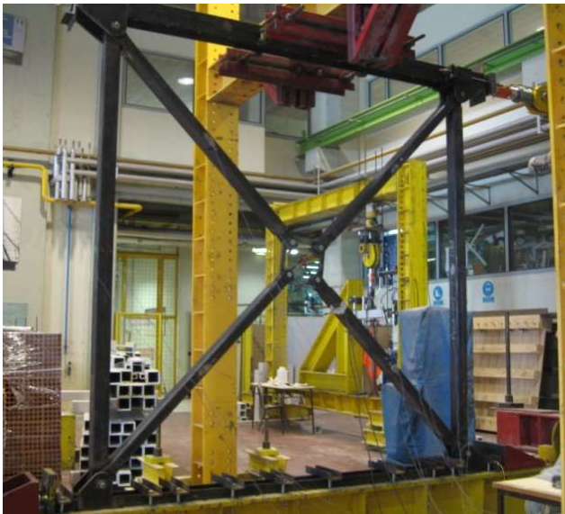
Cyclic test of a full-scale prototype of a Dissipation Panel.
