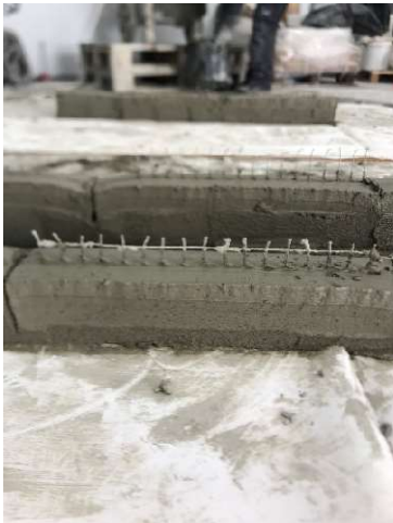
Prototypes of vertical reinforcement.
