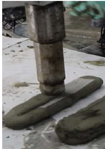
Prototypes of horizontal reinforcement.
