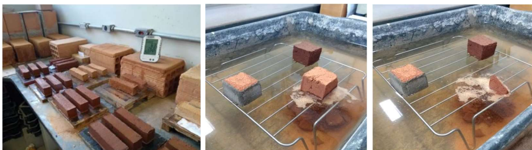
Prismatic and rendering specimens (left) and samples being tested with water; on the right is possible to see how the cow dung addition can improve the water resistance of clay mortars.
