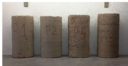
Rammed earth samples for laboratory analysis.
