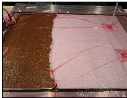
Resin synthesis and FRP composite production using vacuum infusion method.
