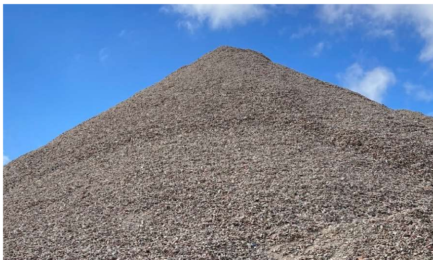
Recycled aggregates produced by a construction and demolition waste operator.
