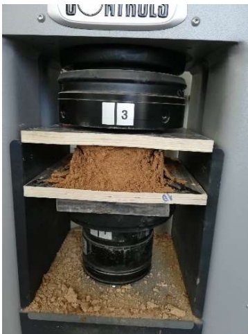
Compressive strength evaluation for a saturated specimen.
