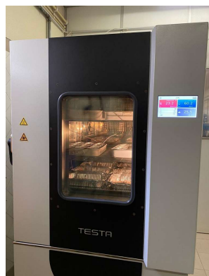
Carbonation chamber TEST/TESCAL CT-TT 300 ECP 20.
