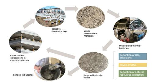
Recycled cement production and use in a closed-circular economy cycle that tackles the main issues faced by the construction and concrete industries.
