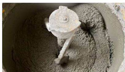
Production of SCC.
