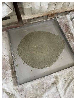
Slump flow and T500 test.
