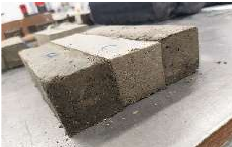
Samples of mortar (fly ash, reference concrete, MIBA).
