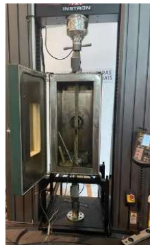
General view of the equipment and instrumentation used for the core material characterization tests, and environmental chamber and universal testing machine.
