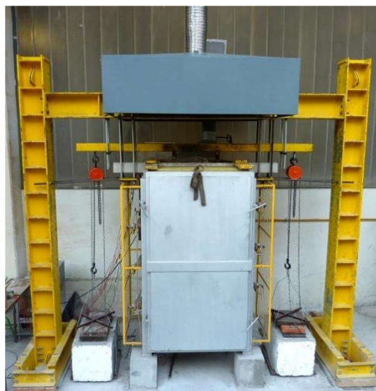
Fire resistance test setup.
