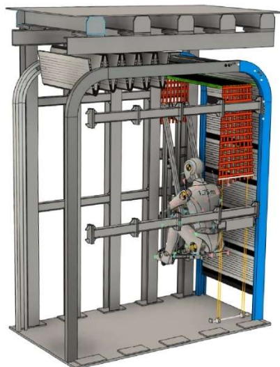
Schematic view of SHELTER (Structural Hyper-resisting Element for Life Threatening Earthquake Risk) with a safety chair and a dummy.
