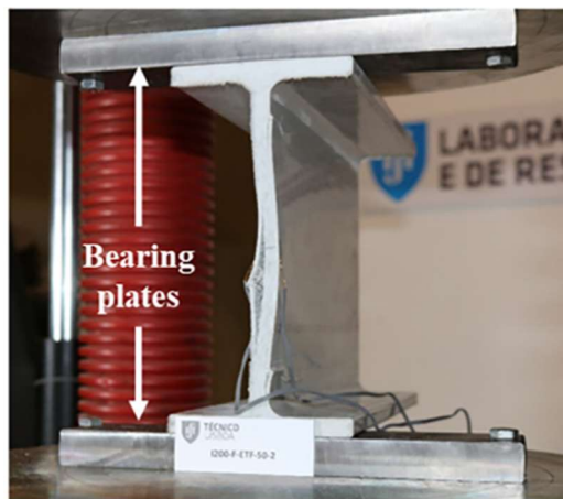
Web-crippling tests setup.
