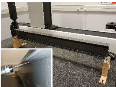
General view of the 3D contact coordinate-measuring machine (CMM) for measurements of the geometrical imperfection of pultruded GFRP profiles, and some typical critical buckling modes of GFRP profiles modelled in the Finite Strip Computer Application (FStr).
