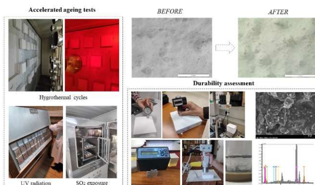
Methodology for the durability assessment of multilayer rendering systems.
