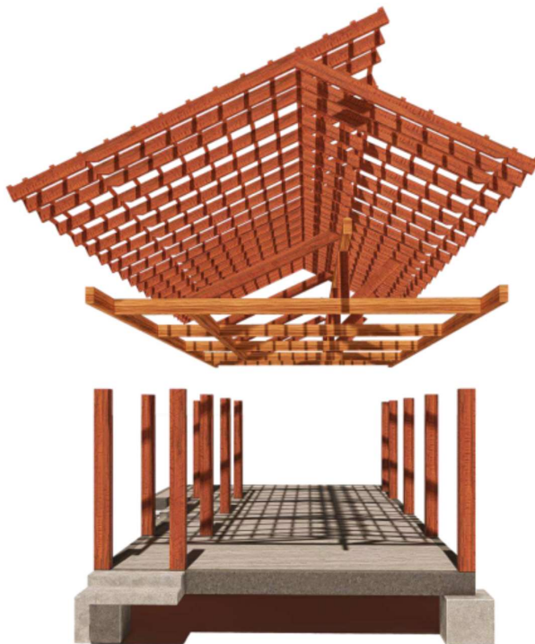
Design of the structural system of the Tekoha o Habitar Indígena project. (Source: Valdomiro).
