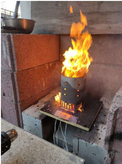
Fire heat flux tests setup.
