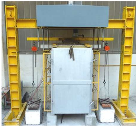
Fire resistance tests setup.
