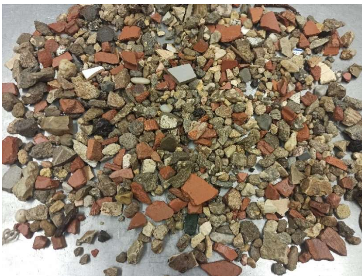
Samples of construction and demolition waste as coarse recycled aggregate.
