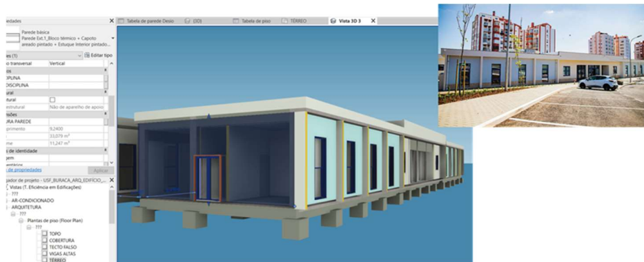
Model with parametric information for QTO automation similar to the real thing - REVIT software.
