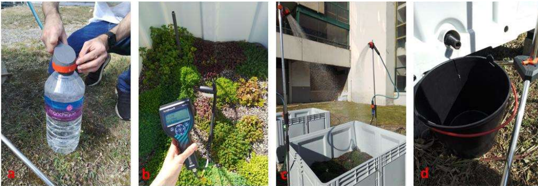
Experimental trials on small-scale green roofs. Runoff measurement (a), substrate moisture measurement (b), artificial precipitation simulation (c), roof runoff collection (d).
