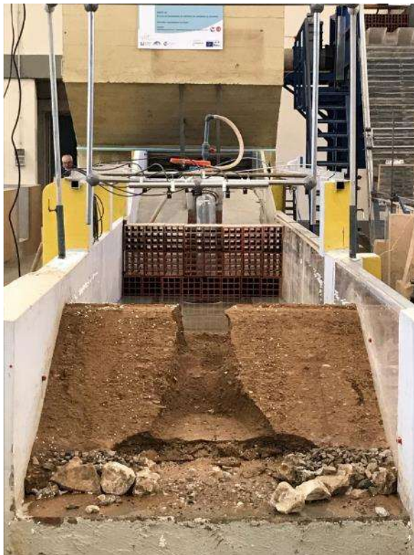
Dam breach by overtopping. Experimental test.
