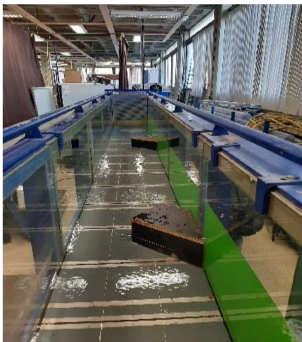
45° flow-refuge configuration (facing downstream) tested at the indoor flume located at the Laboratory of Hydraulics at IST.
