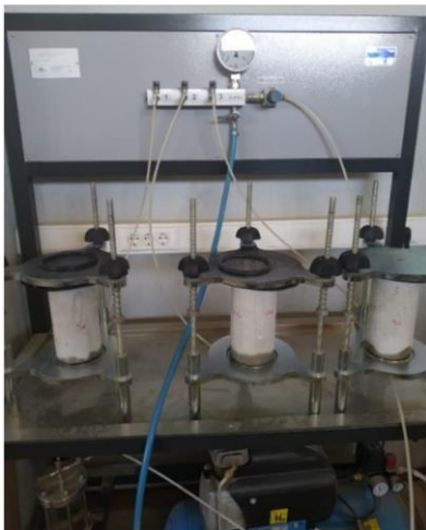
Figure 1. a) Water penetration under pressure test; b) penetration depth in a recycled concrete specimen with treated surface with a bioproduct produced based on mixed microbial cultures from pinewood waste [Serrano-González et al., 2021 - https://doi.org/10.3390/ma14216545 ].
