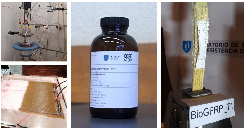
Figure 1. Left to right and top to bottom: reactor for resin synthesis; vacuum infusion of a GFRP plate using a bio-based unsaturated polyester (UPE) resin; bio-based UPE resin; GFRP bio-composite in a tensile test.
