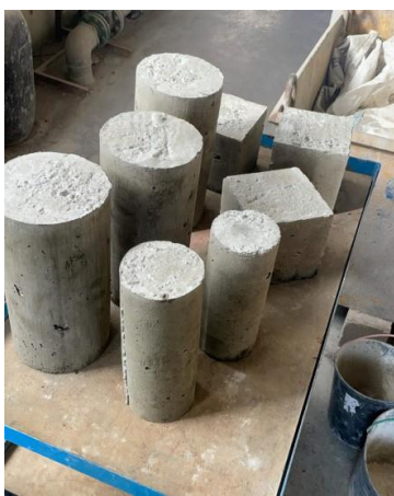
Figure 1. Laboratorial study of concrete with recycled aggregates.
