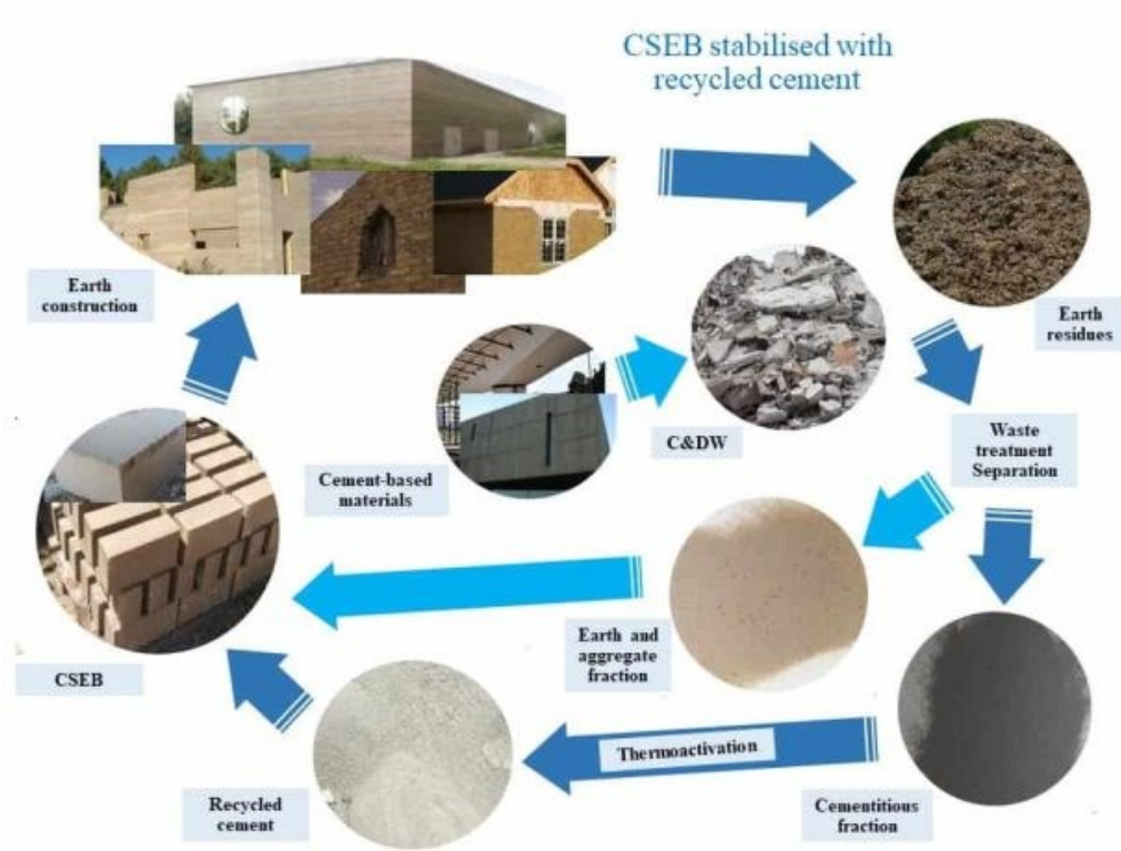
Figure 1. Closing loop of production and recycling of compressed stabilised earth blocks (CSEB) with recycled cement.
