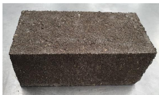
Figure 4. MIBA pavement block according to EN 1338.
