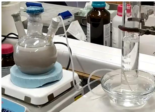
Figure 2. NaOH-based pretreatment of MIBA.
