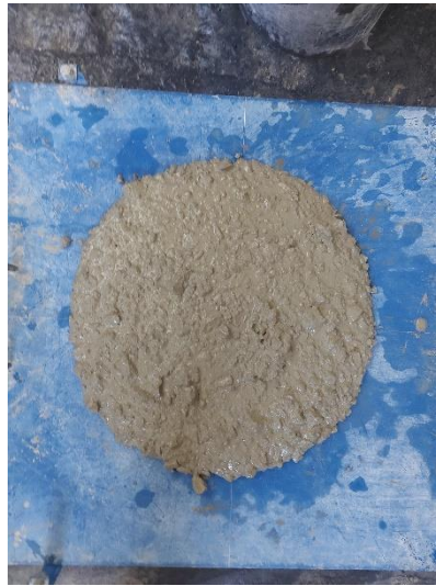
Figure 1. Fresh state tests of recycled aggregate concrete.
