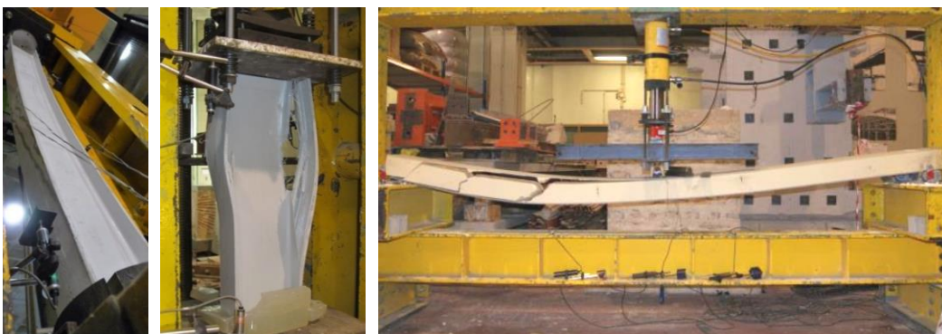
Figure 3. Structural tests (left to right): flexural buckling of pultruded columns, local buckling of pultruded columns, shear failure of sandwich panel.
