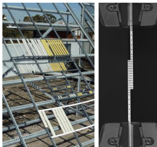
Figure 2. GFRP laminates and adhesively bonded joints placed in the rooftop of LNEC subjected to natural ageing conditions (left) and single lap shear test (right).
