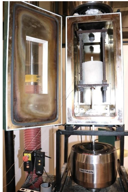
Figure 1. GFRP-concrete bond tests setup.
