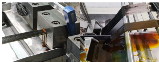
Figure 3. Pilot production of pultruded CFRP bio laminates using the BUPE1 resin.
