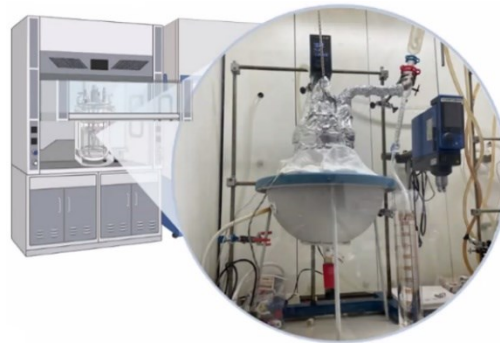
Figure 2. Reaction system to synthesize the BUPEM resin.
