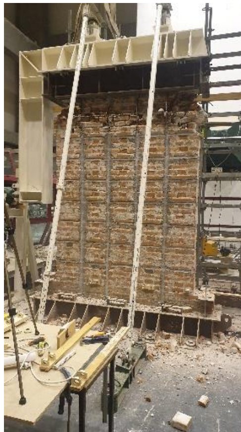
Figure 1. Full-scale reinforced wall test on the seismic table.
