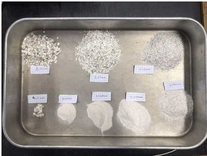
Figure 2. Distribution of different particle sizes of oyster shells waste.
