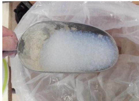
Figure 1. Aspect of the lightweight insulation aggregates used - silica aerogel.
