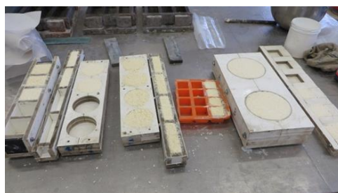
Figure 2. Used frames for the initial tests made to the different thermal render compositions studied.
