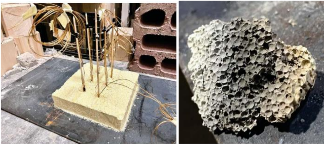
Figure 1. EPS Mortar testing set-up (on the left) and detailed view post-exposure to standard fire curve (on the right).
