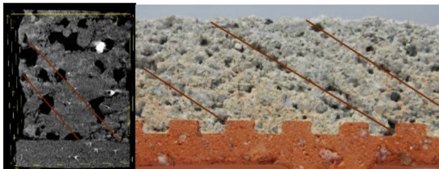
Figure 2. On the left: Micro-CT section; on the right: cross section of applied mortar on brick substrates.
