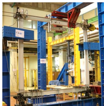
Figure 3. 2D frame sway tests.
