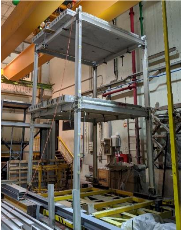
Figure 4. 3D frame shaking table tests.
